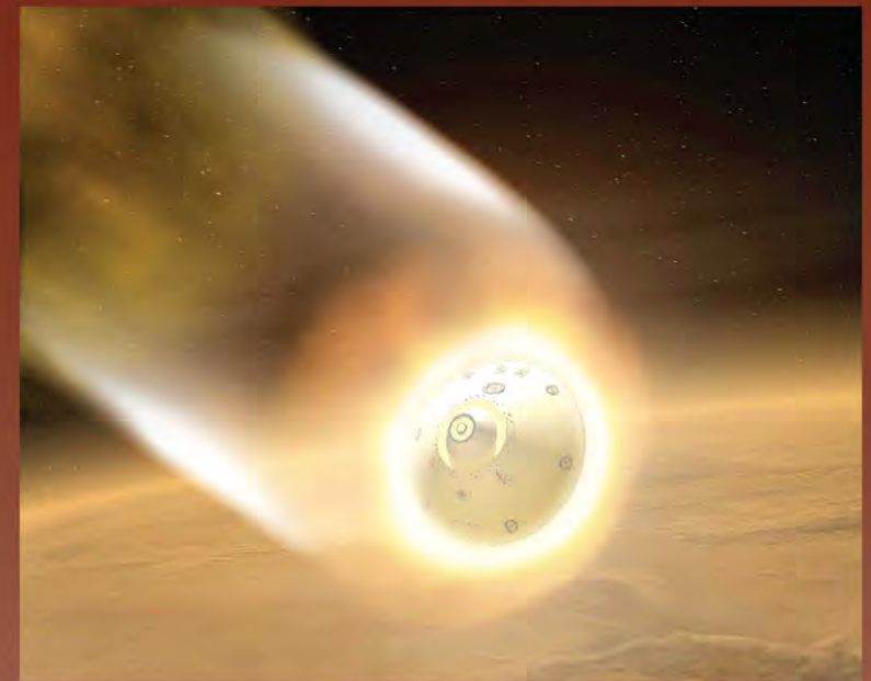
The aeroshell protects the rover from fiery temperatures as it enters the Martian atmosphere. (Artist's rendering)
